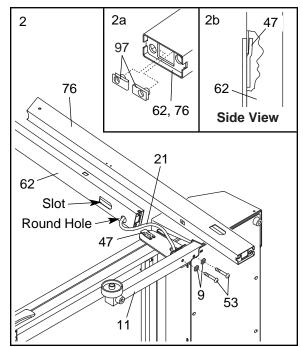
3. With the help of a second person, tip the treadmill so the Base Pads (40) (see drawing 1) are laying flat on the floor. Rraise the Uprights (62, 76) to the vertical position.
